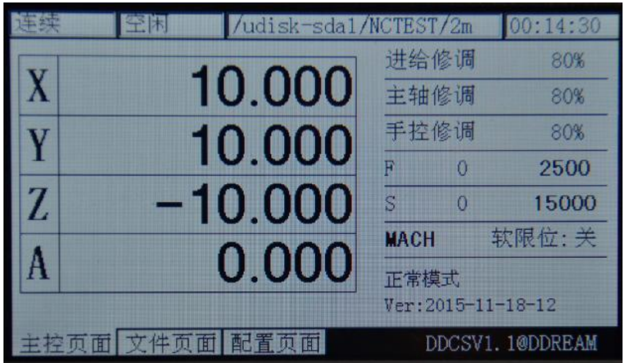
Picture3-62. Switch to the machinery coordinate system
