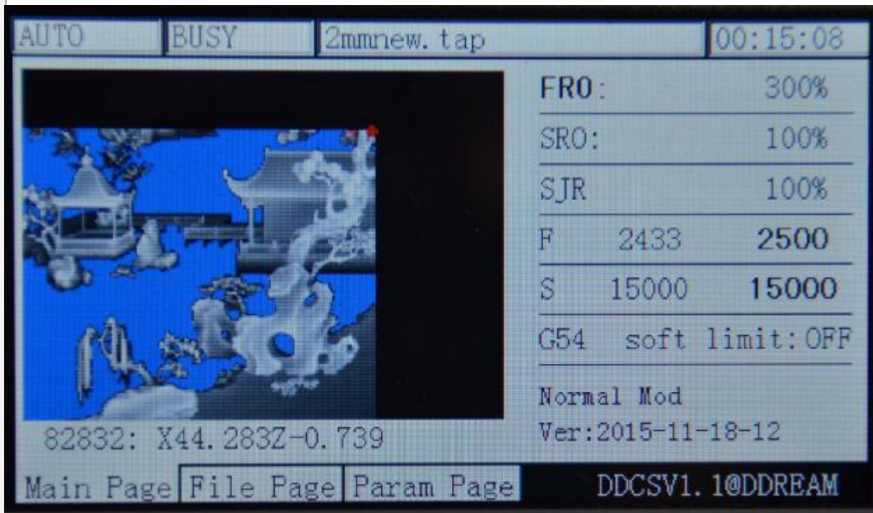
Picture3-15. Tool path display status when the processing is approaching to end
